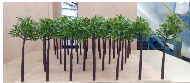
Fig. 5. Tree models used in the flume experiment, and a single tree parameter: height is 20 cm, and the diameter is 0.6 cm.
