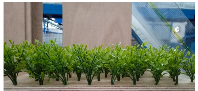
Fig. 7. Shrub models used in the flume experiment.
