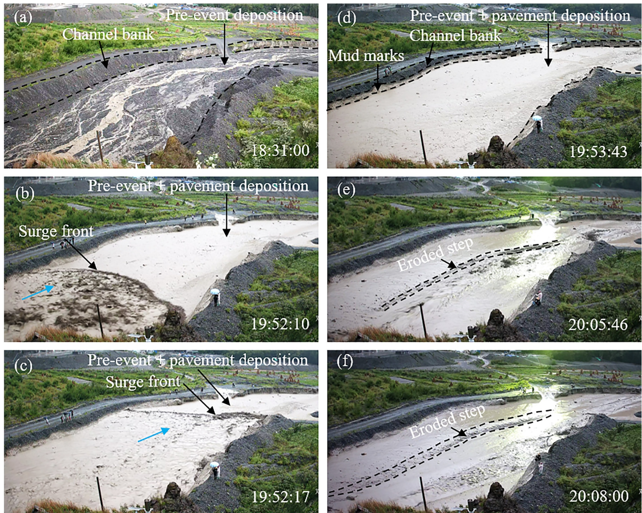
Figure 3. Typical moments of the surge-flow event and channel-bed evolution at the Jiangjia Ravine. (a) Prior to the surge-flow event; (b and c) an approaching debris-flow surge in motion. The direction of incoming flow is from lower left to upper right (the blue arrows). (d) Deposition in the channel after the debris-flow surge in panels (b and c). (e and f) Formation of an eroded step into the pre-event deposition after the surge-flow event.
