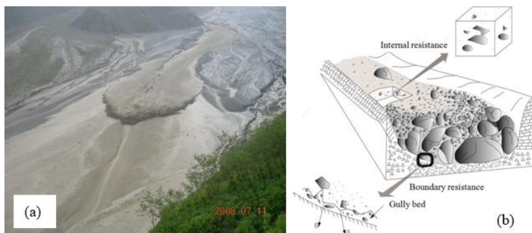
Figure 1. The photo and sketch of debris flow flowing in channel. (a) Debris flow in Jiangjia gully, Dongchuan, China [17]; (b) flow resistance in channel [18].
