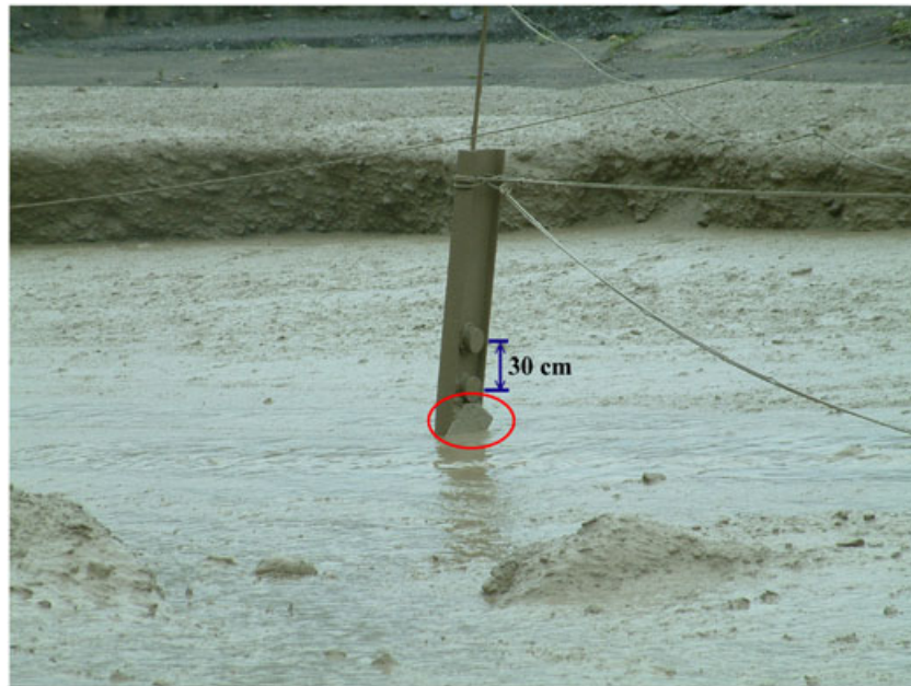
Figure 5. Boulder stopped by the steel pile after debris flow passed by. (The third sensor was covered by slurry and debris deposits. It is easily noted that the bed elevation was changing and higher than that in Figure 2a.). This figure is available in colour online at wileyonlinelibrary.com/journal/espl
