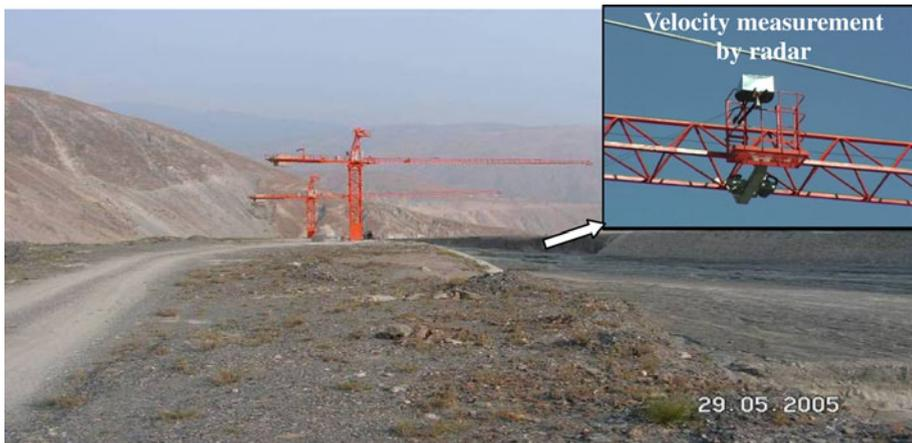
**Fig. 5** The observation equipments for velocity measurement in JJG
