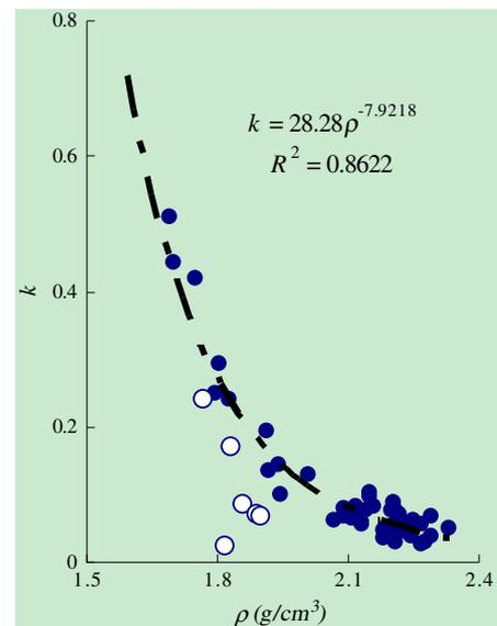
Fig. 6. Distribution parameter varying with debris-flow density.
